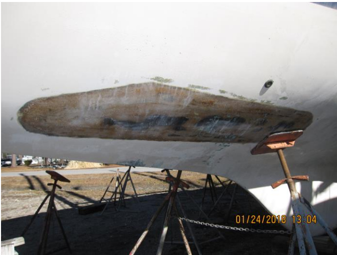
Detail of fiberglass hull repair, port side
