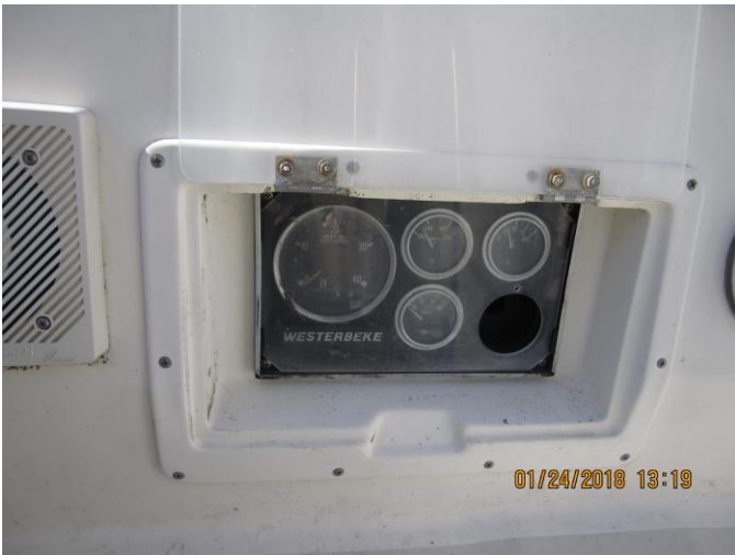
Engine instrument panel and cover to be replaced
