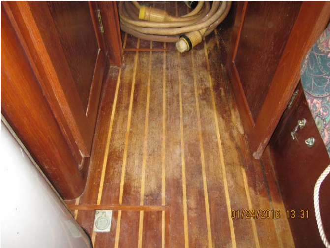
Water damaged cabin sole veneer
