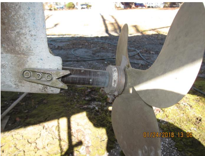
Spurrs line cutter on propshaft needs zincs.
