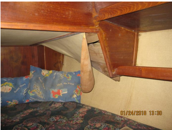
Water damage in quarterberth cabin. All soft goods should be replaced due to mildew/mold
