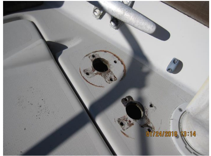
Windlass foot switches missing
