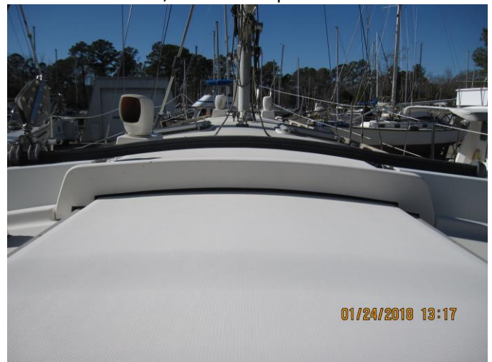
Mainsheet traveler bent upwards gently from loading. May be OK.
